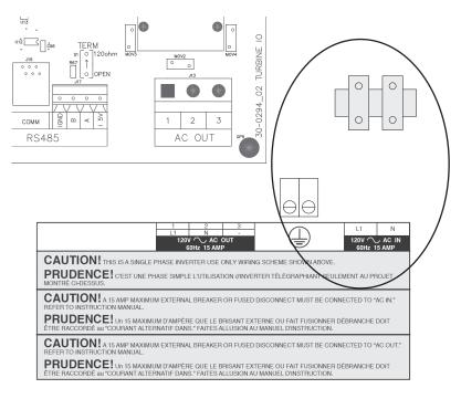
Figure 2.9 AC Input Current Wiring Diagram
